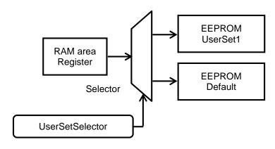
When executing UserSetSave, write the camera setting information from the RAM into the memory area that was selected on the UserSetSelector. Note: UserSetSave is not available when Default on UserSetSelector was selected.
