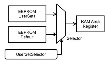
When executing UserSetLoad, write the camera setting information from the RAM into the memory area that was selected on the UserSetSelector.
